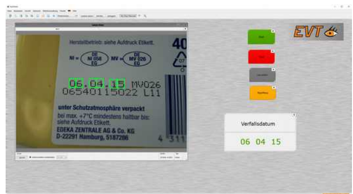
EyeVision Process Mode: expiration date inspection
